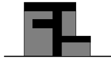
Figure 4.1: Illustration of the “filled” and “shade” fitness function. The structure itself is black. The filled fitness measures union of both back and grey regions, the shade fitness measures only the grey area.
