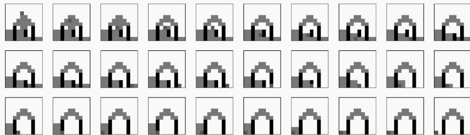
Figure 5.6: Robust Assembly Plan Frames 50-80: scaffolding is removed
