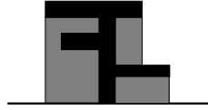
Figure 5.10: Illustration of Shaded Fitness Function. The structure itself is black, and the gray region is considered “shaded”.
