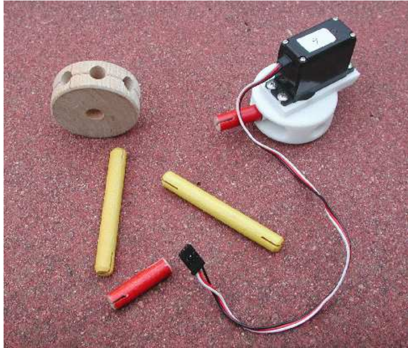
Figure 4.4: Basic building blocks of the system: rods of regular length and fixed and actuated joints.
