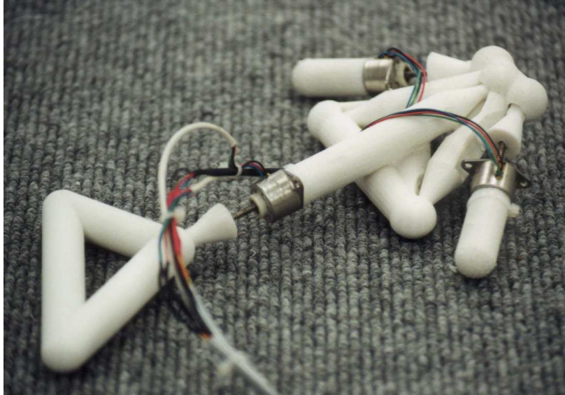
Figure 2.34: Walking robot evolved by Lipson and Pollack builds further on our paradigm of evolution of structure under buildability constraints, adding movement and control.
